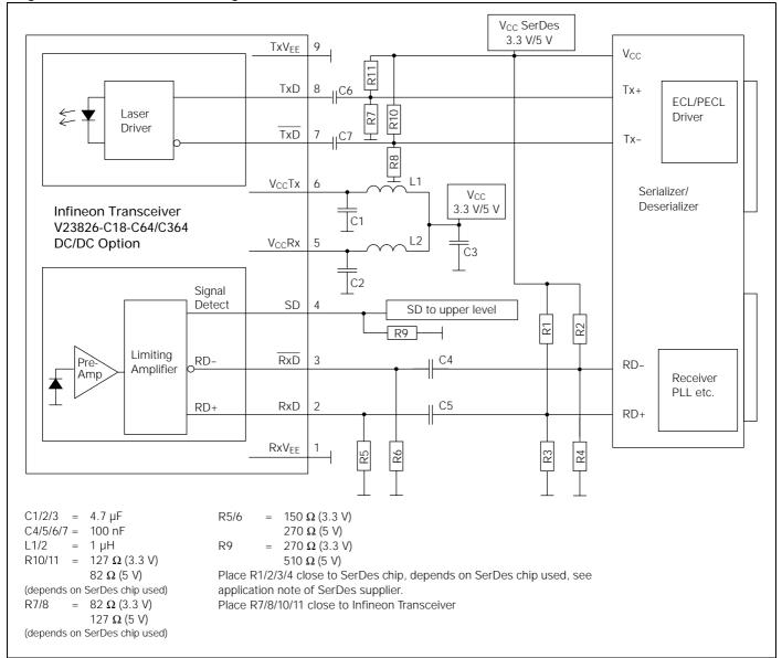
This Application Note assumes Fiber Optic Transceivers using 5 V power supply and SerDes Chips using 3.3 V power supply. It also assumes no self biasing at the receiver data inputs (RD+/RD-) of the SerDes chip (Refer to the manufacturer data sheet for other applications). 3.3 V-Transceivers can be directly connected to SerDes-Chips using standard PECL Termination network.
